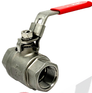
FIG. S-292T / C-292T: THREADED ENDS, ¼" TO 2": 2000 W.O.G., 2 ½" TO 4": 1500 W.O.G.
