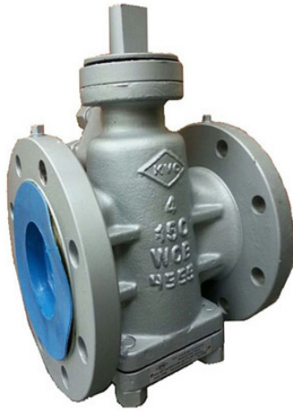
FIG. 282-CS-150 CLASS 150 FLANGED ENDS BOLTED BONNET WCB BODY & BONNET 13Cr/HF TRIM
