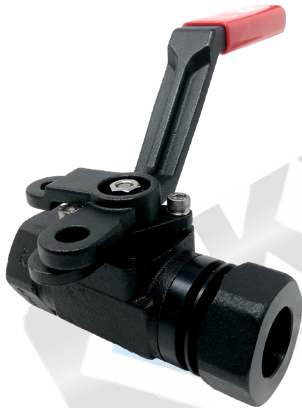
FIG. C-336SS-LF2: 6000 WOG CLASS 2500 EXTENDED SOCKET WELD X SOCKET WELD ENDS ¼" TO 1 ½": FULL PORT, 2": STANDARD PORT ISO 5211 MOUNTING PAD NACE MR-01-75
