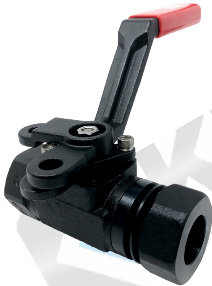
FIG. C-333ST-LF2: 3000 WOG CLASS 1500 EXTENDED SOCKET WELD X THREADED ENDS NACE MR-01-75 1/4" to 1 1/2": Full Port 2": Standard Port, ISO 5211 Mounting Pad
