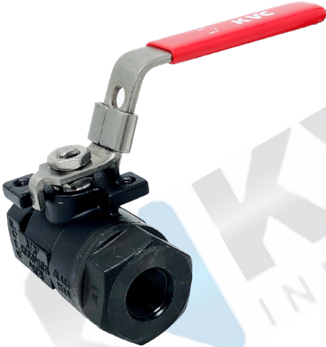
FIG. C-206TWL-F: 6000 WOG, ¼" TO 1 ½": FULL PORT, 2": STANDARD PORT THREADED ENDS, NACE MR-01-75 ISO 5211 MOUNTING PAD LEVER HANDLE FIRE SAFE
